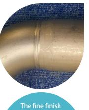
of the weld (above) is obtained by TIG welding method (below). The smooth bead (welded area) is vital for the water flow
